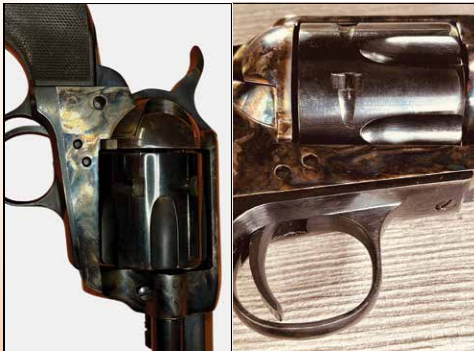
THE CYLINDER NOTCHES ARE LENGTHENED TO A POINT INSTEAD OF ROUND FOR SMOOTHER ROTATION OF THE CYLINDER.
