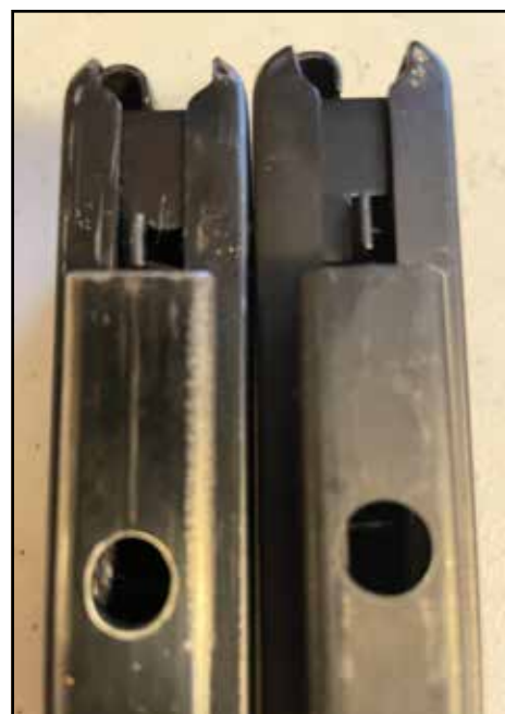
L-R: ORIGINAL SUBMACHINE GUN 30-ROUND MAGAZINE WITH ¼-INCH MODIFICATION VS. T-RIFLE 30-ROUND MAGAZINE.
